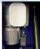
2. Motor, Springs, Limited Switch (Work Strong + Stable Working)
